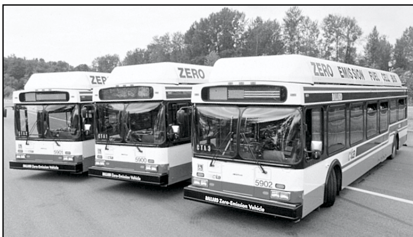
2nd Generation Fuel Cell Transit Buses in Chicago Source: Ballard Power Systems
